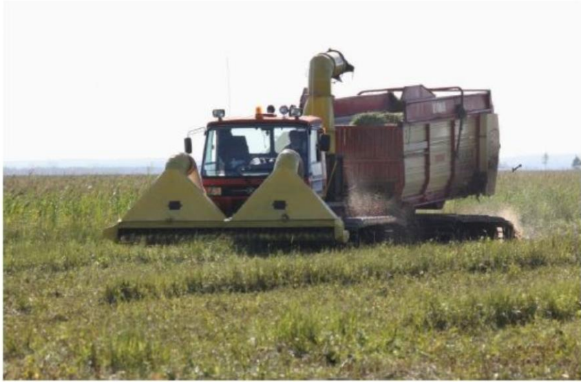
Fig. 2. Tracked mower developed from a modified snow groomer (photo by Piotr Marczakiewicz).
